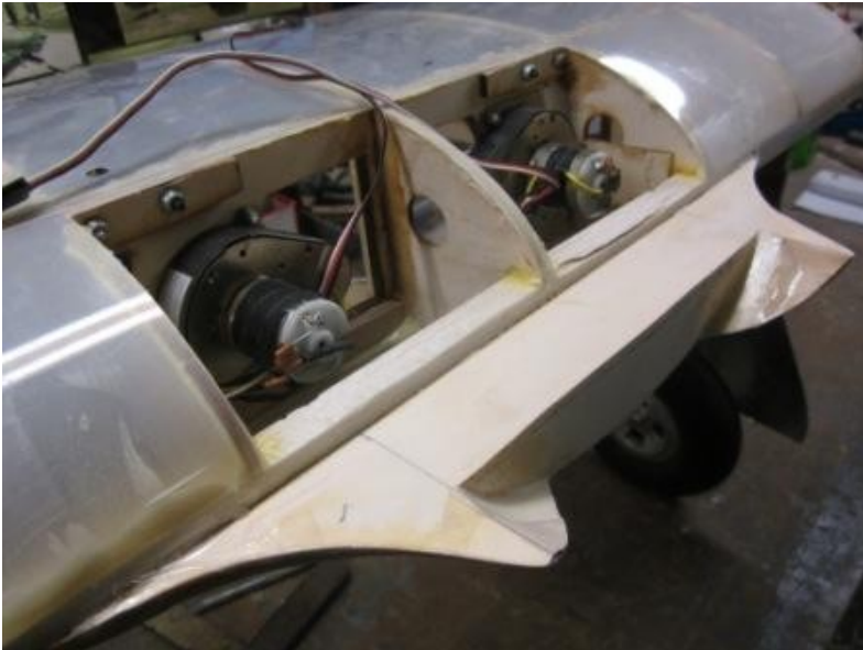
Finished front fairing from the topside of the centre wing section.
